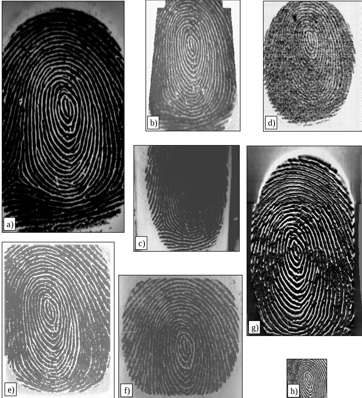
a) Biometrika FX2000, b) Digital Persona UareU2000, c) Identix DFR200, d) Ethentica TactilSense T-FPM, e) ST-Microelectronics TouchChip TCS1AD, f) Veridicom FPS110, g) Atmel FingerChip AT77C101B, h) Authentec AES4000.
